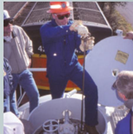
*BNSF's Pat Brady demonstrates the fine points of a pressure tank car gaging rod. Through the use of air and water on the training cars, responders can better visualize what types of leaks they could be faced with.*
