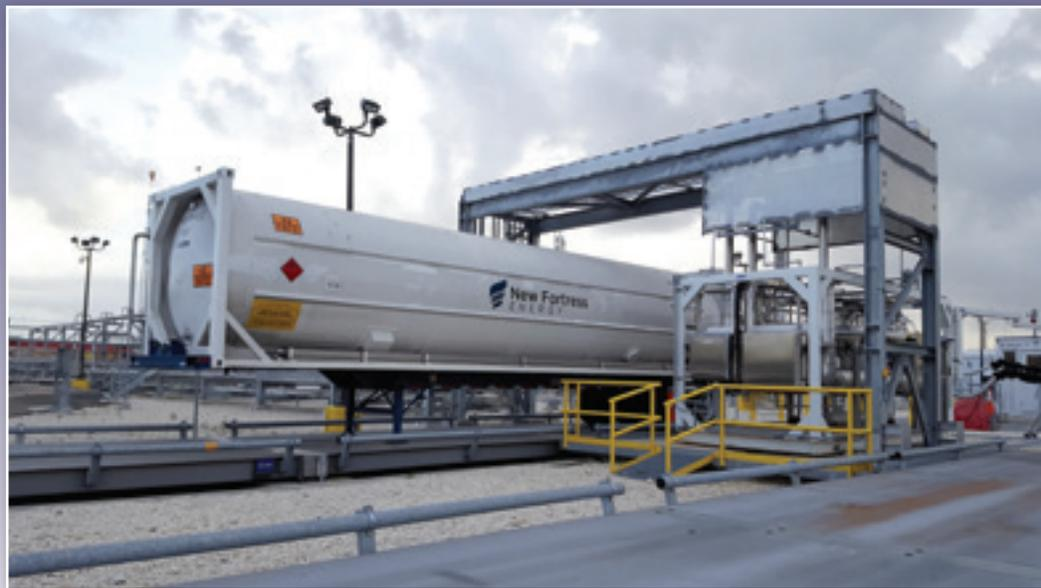
exported to the Caribbean from the operational liquefaction facility located in South Florida through the Port of Miami via ISO containers.
