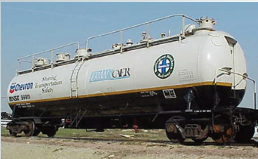
The centerpiece of BNSF's hazmat training props (ca. 1999) between classes in Rancho Cucamonga, CA. Note the added end door that made for easier entry. Photo: Brock Lowman
