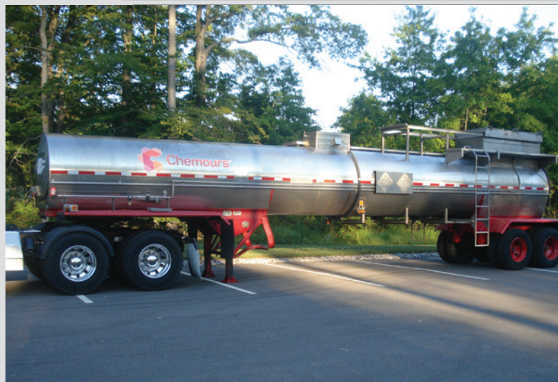
Chemours training unit tanker for Sulfuric Acid.
