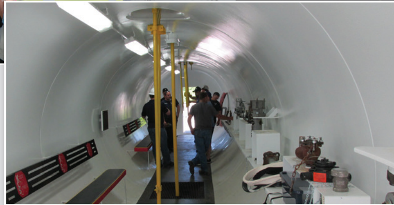
The KCSR HazMat training tank car classroom is outfitted with training tools to acquaint emergency first responders with equipment they might encounter when responding to a rail emergency. Photo by Gary Johnson, Transportation & Industrial Services, Inc.
