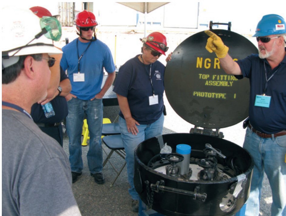
Roar Brock of Midland Manufacturing discusses the differences in the new dual-valve system as compared to the traditional chlorine valve arrangement
