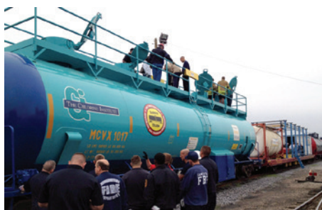
Louisville 2015: During the Tank Car 101 Workshop, Barry Draffen (Westlake Chemicals) describes the different types of protective housings and fittings on top of MCVX 1017, while Thomas Clifton (Paducah & Louisville Railway) covers the basics of tank car anatomy on the ground.
