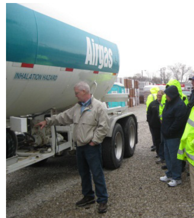
Dave Point of AirGas explains the Emergency Shutdown valves on the MC-331 cargo tank.
