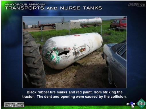
10. The gash, tire marks, and the red paint all were from the collision with the tractor
