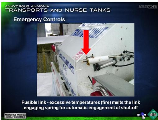
d. This is an example of a fusible link. In case of fire, the fusible link would melt and either activate a spring that would expand and engage the lever or would release air, actuating the shut-off
