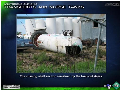
11. The missing shell section remained by the load out risers
