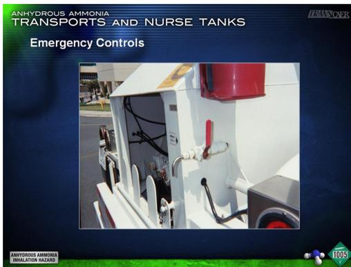
c. Air activated remote shut-off at the rear passenger side. Flip the red handle down and air would be released closing the internal valve
