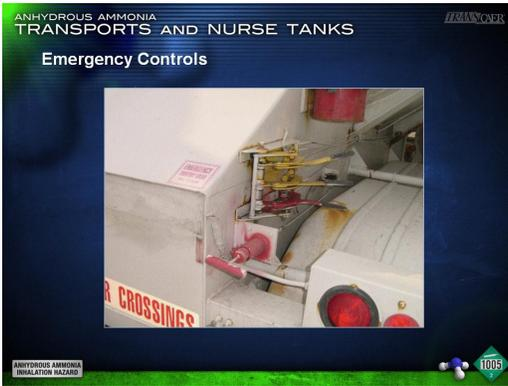
b. Rear passenger side remote shut-off is cable operated, you would pull the red handle out to actuate it
