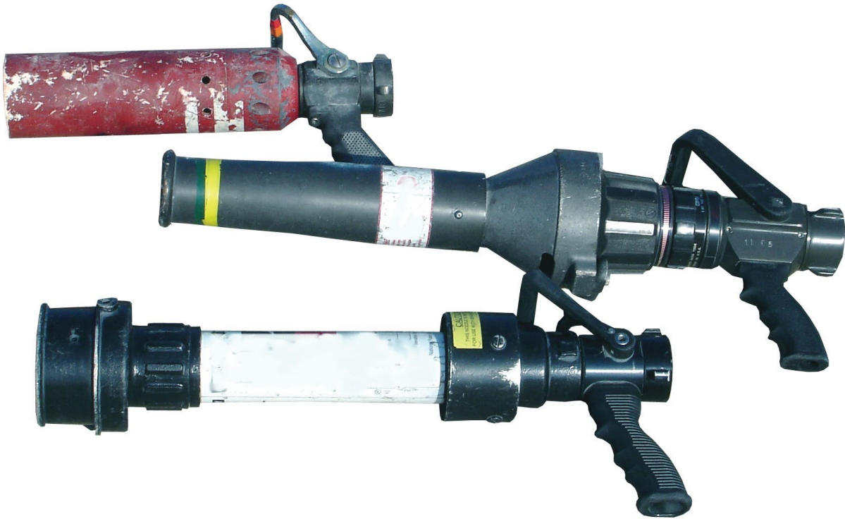
Figure 6.6: Air Aspirating Nozzles
