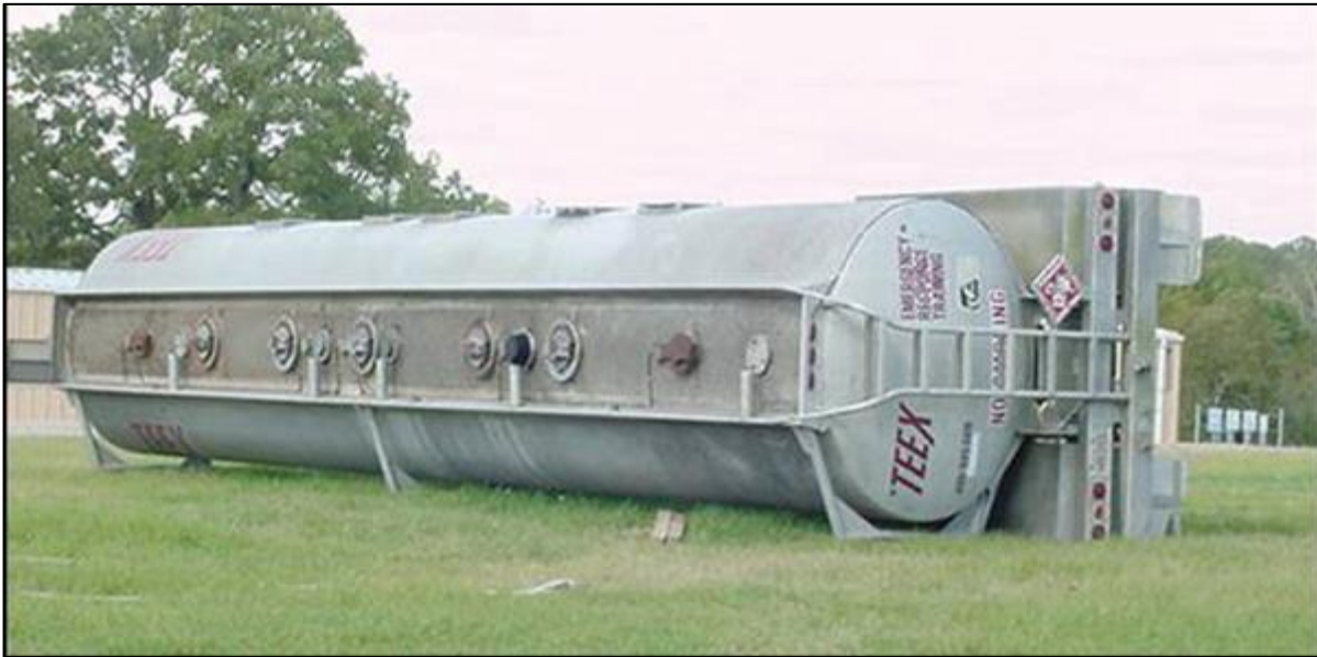
Figure 4.6: Overturned MC-306/ DOT-406 Cargo Tank
