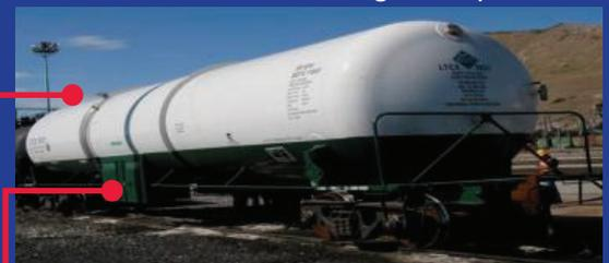
Refrigerated liquid - Argon most common - venting from pipes up the side of the car is normal operation.
