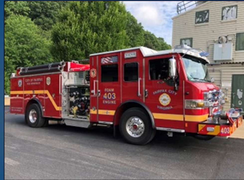
300 gal. AR-AFFF & 600 gal. water
