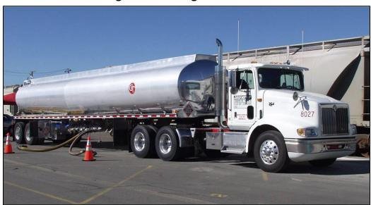
Figure 4.10: Cargo Tank Truck
