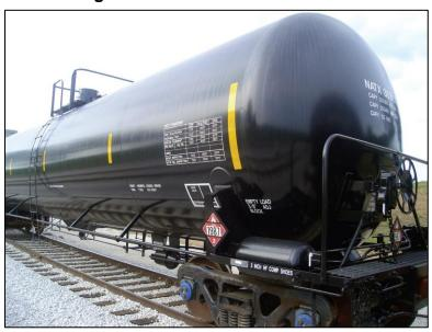
New regulations for rail tank cars construction were published in 2015. New rail tank cars constructed after October 1, 2015 are required to meet enhanced DOT Specification 117 design or performance criteria. Existing rail tank cars must be retrofitted by 2023 in accordance with the DOT-prescribed retrofit design or performance standard.
