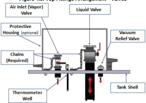
Figure 4.8: Top Fittings Arrangement—Valves
